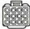
MOLEX FEMALE CONNECTOR RECEPTACLE 2 PIN .093-380189 3 PIN .093-380035 6 PIN .062-380107 9 PIN .062-380109 12 PIN .062-380111 2 PIN .093 INTL-380280 3 PIN .093 INTL-380288 4 PIN .093 INTL-380293 6 PIN .093-380037 9 PIN .093-380039 12 PIN .093-380041
